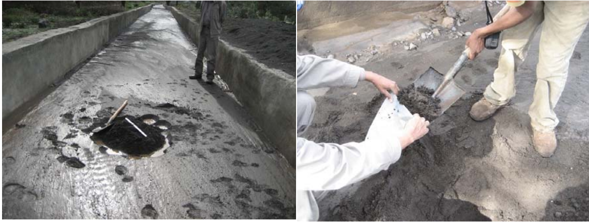
Figure 31. Pictures showing sediment data collection by the method of grab sampling taken by shovel
